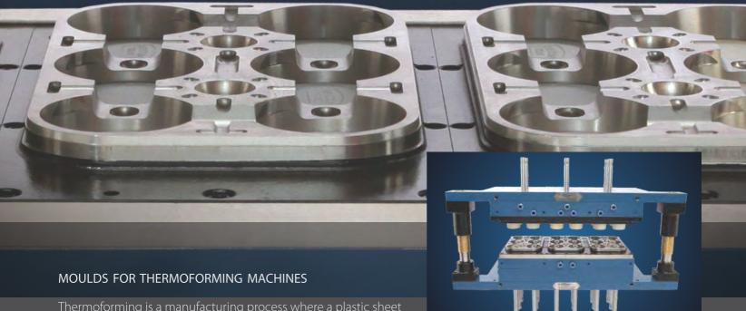
Thermoforming is a manufacturing process where a plastic sheet is heated to a forming temperature, formed to a specific shape in a mould and trimmed to create a usable product. The sheet or "film" when referring to thinner gauges and certain material types is heated to a high-enough temperature so that it can be stretched into or onto a mould and cooled to a finished shape.
